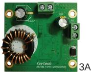
With this DC-DC Converter you are able to make your faytech device compatible for varying power inputs from 9-36V.
